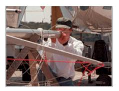
pulling hard enough on the forward lever to bring the spreaders back to their stops. Check to see if they hit simultaneously. The mast manufactures usually do a good job with these measurements but they can change over time.
